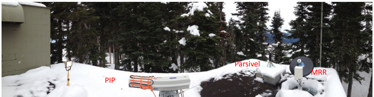
Figure 11: The suite of instruments installed at Hurricane Ridge on the north side of the Olympic Peninsula. They include a PIP, MRR, Parsivel and Hot Plate (not shown).
