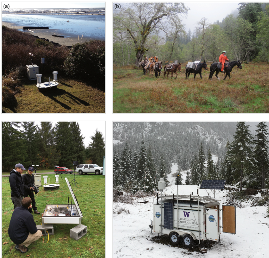
FIG. 3. Examples of the OLYMPEX surface observation sites. (a) Beach House site on the coast. (b) Mule train taking instruments to remote higher-elevation sites. (c) Installation of 2DVD (foreground) at the Fisheries site; dual-platform tipping-bucket gauge and Parsivel disdrometer are in the background. (d) University of Washington mobile trailer facility in the Wynoochee drainage. Photo credits: (a) Lynn McMurdie, (b) William Baccus, and (c),(d) Joe Zagrodnik.
